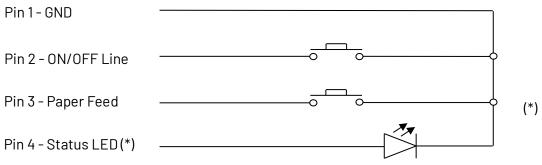
A serial resistor (180 ohms) is on the printer, setting the LED current at about 5mA. In addition, an on-board status led is also present near power supply connector.
